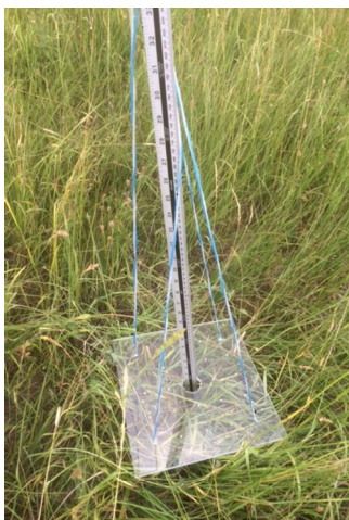
Falling plate meter in the field
